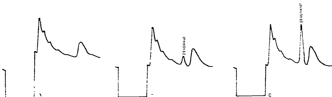
Fig. 1. Chromatogram obtained on a column packed with Ultrabond 20M (100–120 mesh). (A) 12.5 mg of cauliflower; (B) 12.5 mg of cauliflower fortified with 0.02 mg/kg of propoxur; (C) 12.5 mg of cauliflower fortified with 0.1 mg/kg of propoxur.
